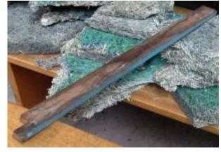
material could have led to sudden facture. Once a piece of woodwool fractured there would be nothing underneath to keep it up in the lantern and it and everything else unsupported around it would then fall to the ground.
