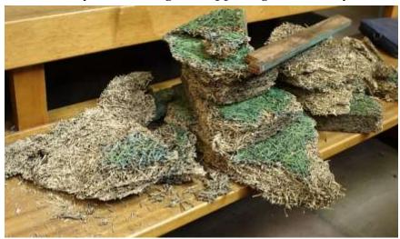
The large pieces of woodwool which fell out of the lantern stacked on a bench after the event. The water stained wooden spacer which also fell showed a vital clue to damp having been present up there.
